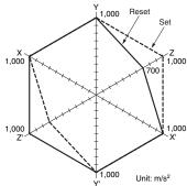
Sample: G6BK-1114P-US Number of Relays: 12 pcs Test Conditions: The value at which malfunction occurred was measured after applying shock to the Shock direction test piece 3 times each in 6 directions along 3 axes.
