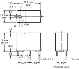
Dimensions in pointed brackets < > are for the Relay mounted to Socket.
